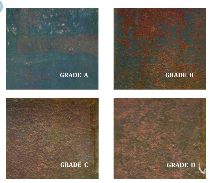
**Grade A** Steel surface largely covered with adhering mill scale but little, if any rust. **Grade B** Steel surface which has begun to rust and from which the mill scale has begun to flake. **Grade C** Steel surface on which the mill scale has ruted away or from which it can be scraped, but with slight pitting visible under normal vision. **Grade D** Steel surface on which the mill scale has rusted away and on which general pitting is visible under normal vision.
