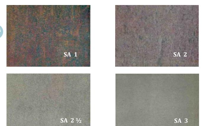
**Sa 1 Light blast -cleaning** When viewed without magnification, the surface shall be free from visible oil, grease and dirt. And from poorly adhering mill scale, rust, paint coatings and foreign matter.
